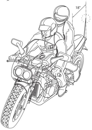
A minimum distance of 18" between the CB antenna and the operator or passenger of the motorcycle should be maintained.
